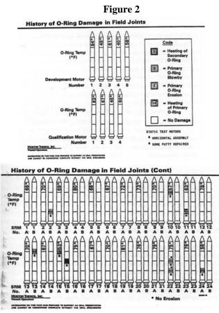
**Figure 2:** Bad data presentation of O-ring failure of previous shuttle flights. Cryptic icons and chronological organization obscure relevant relationships between temperature and O-ring failure.
